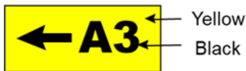
Figure 8.98 (2) Runway exit sign (illustrates matters)
