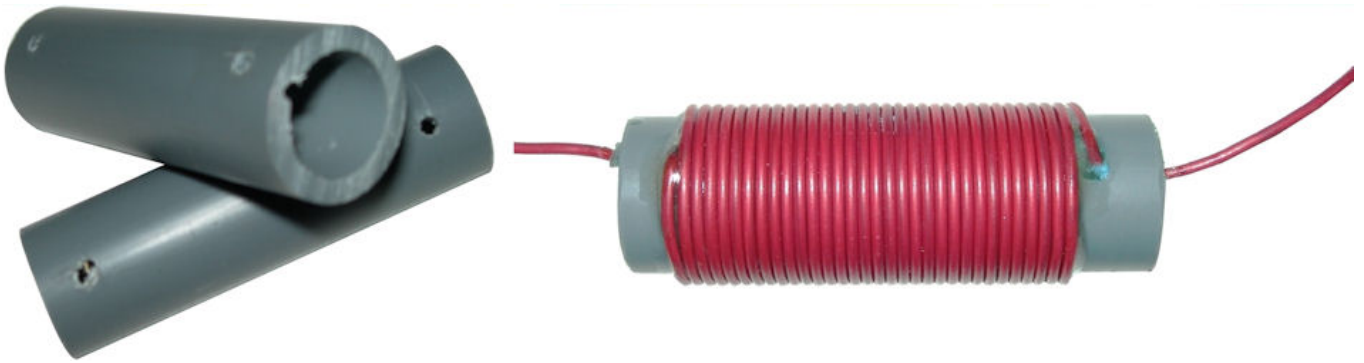
Figure 7: Two blank PVC coil cores and a finished 32-turn coil (notch of groove is visible in top blank core)
