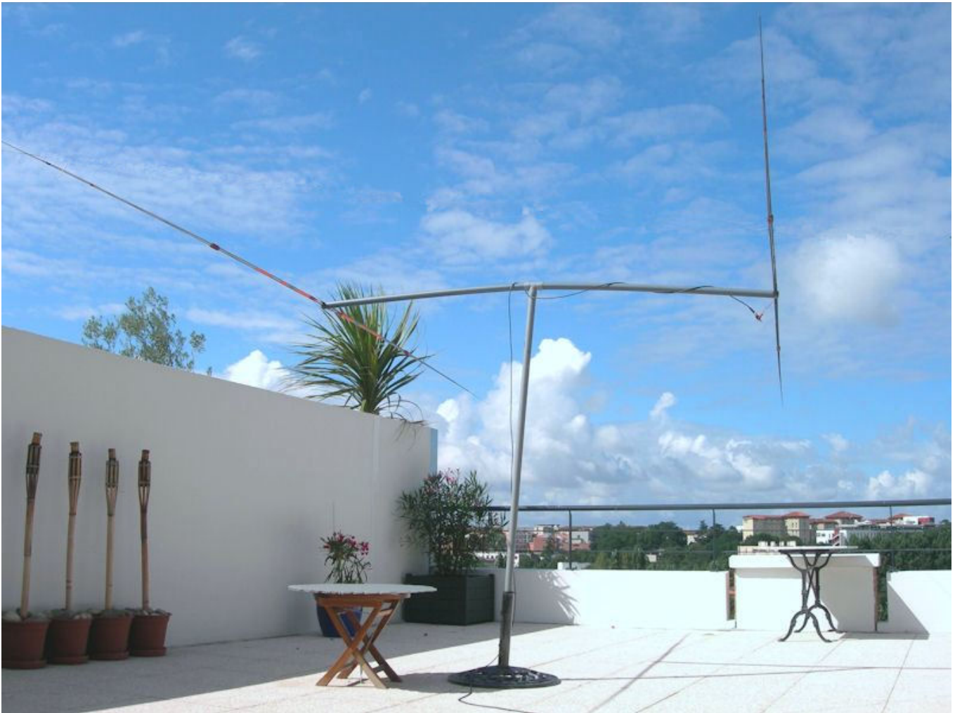
Figure 12: My first Yagi, fully assembled and installed
