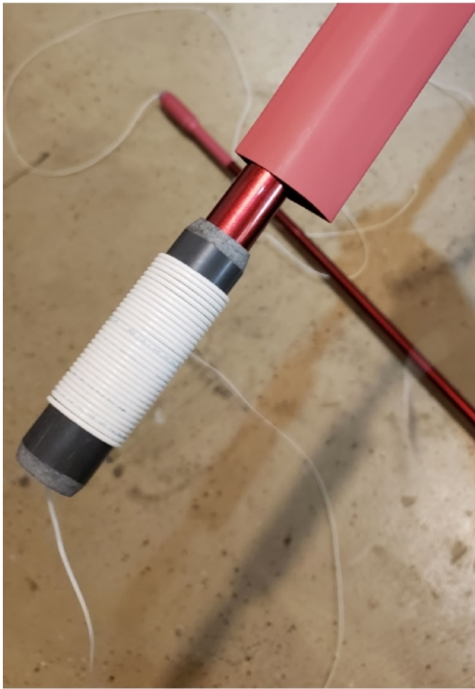
Figure 15: One of Nick's loading coils and SWR reading (photo ©2019 KE4ZMY, used with permission)
