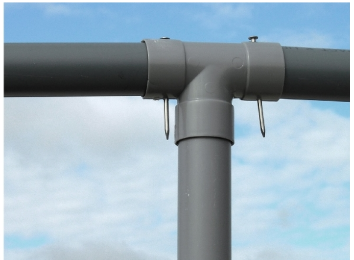
Figure 10: Close-ups: quick-disconnect of the reflector and T-joint of the PVC boom and mast
