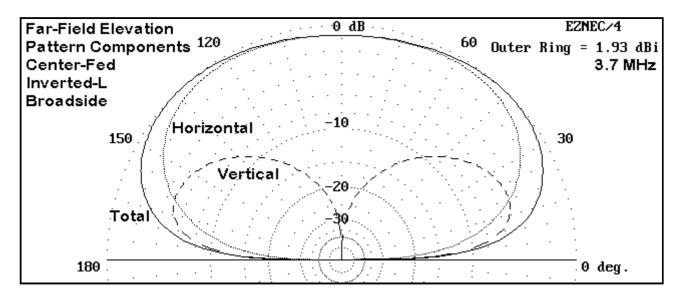
The elevation pattern above shows the vertical, horizontal, and total field components of the inverted-L radiation pattern taken broadside to the horizontal arm of the antenna, where radiation is strongest. In the plane off the ends of the horizontal arm, horizontally polarized radiation is somewhat weaker, but the vertically polarized radiation remains at full strength, with some pattern bending away from the horizontal arm.
