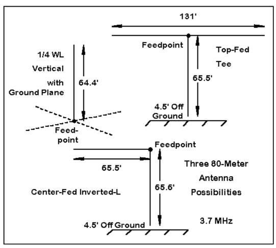
Each antenna was modeled using #14 copper wire and average ground throughout. Note that the inverted-L and the T present challenges to the builder in terms of routing the parallel feedline to the top feedpoint. We shall do some comparisons, but first, let's become a bit more familiar with the inverted-L basic pattern.
