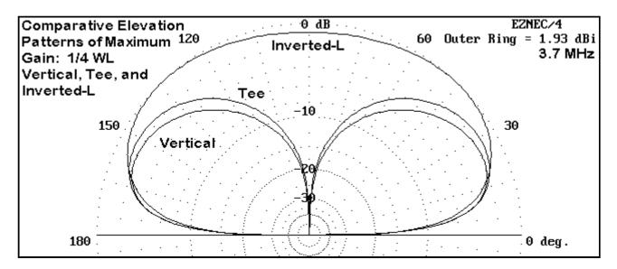
The comparative pattern above shows the rough equality of the T and the ground-plane-vertical patterns under the specified conditions. Surprisingly, the inverted-L comes close to both antennas in low angle radiation. It also has stronger high angle radiation--without becoming a cloud burner--which is useful for shorter skip contacts. In other words, the inverted-L has potential as an all-purpose low-band antenna.
