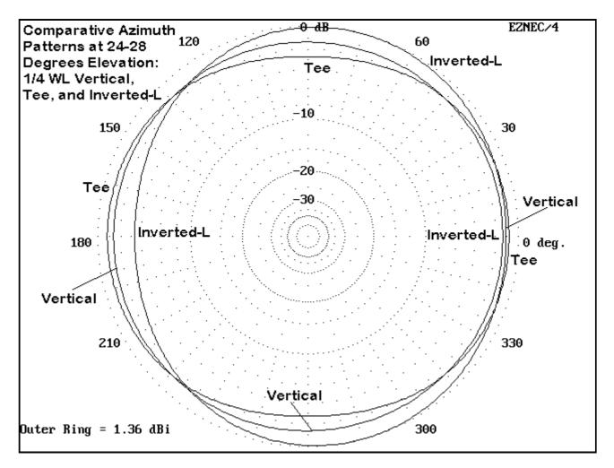
The azimuth patterns of the three antennas--taken at elevation angles between 24 and 28 degrees--show the slight oval of the T and the slightly more radical oval of the inverted-L. The L's azimuth pattern also shows the slight displacement in the direction away from the horizontal arm.
