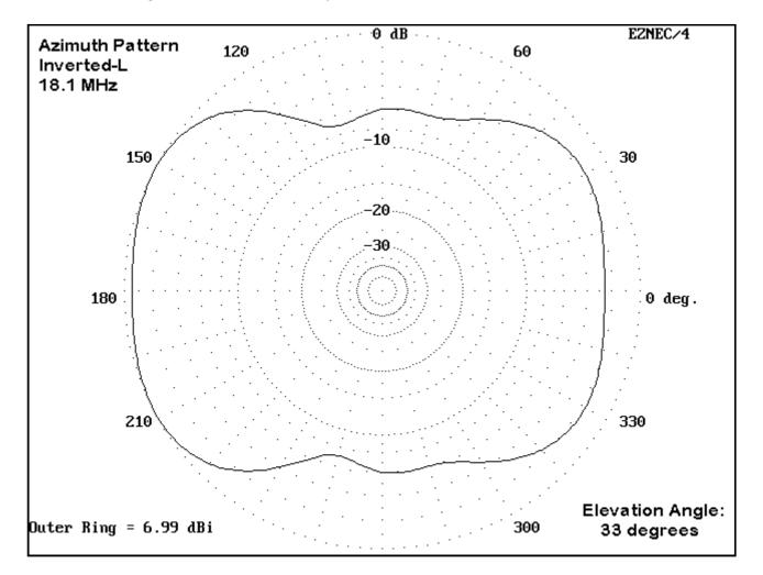
The annotation "square" to describe the azimuth pattern is illustrated by the 18.1 MHz pattern. On this band, the strongest signal occurs at the second elevation lobe. There is a usable but less strong lobe at about 16 degrees elevation. Note the absence of sharp nulls and lobes.
