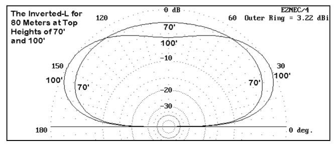
The elevation patterns in the figure compare the antenna at 70' and at 100' and add visual confirmation of the conclusion drawn from the table.
