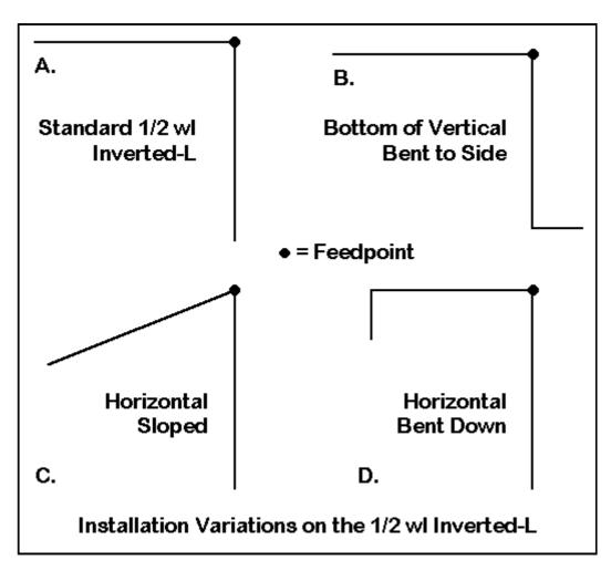
*Bending the vertical at the bottom*: The first way to save vertical space or to protect family members from the high voltage at the antenna element end is to bend the lower end of the vertical to the side. The upper horizontal arm remains 65.5' long. The overall length of the vertical is also 65.5', but part is now vertical and part horizontal. I tested three scenarios, listed in the table below:
