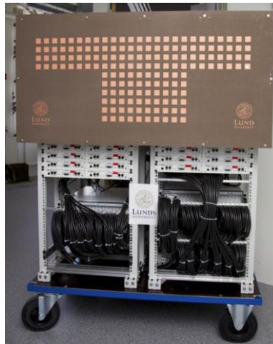
Fig. 2. One of the World’s First Real-Time Massive MIMO Testbeds - Created at Lund University Using the Massive MIMO prototyping system [2]
