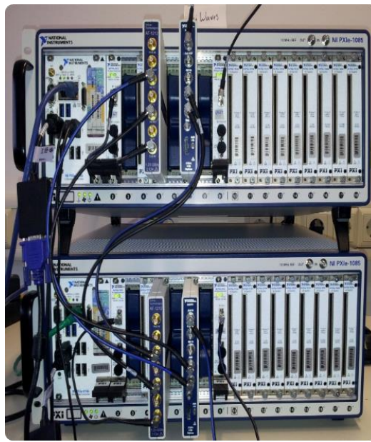
Fig. 4. Baseband prototype system for mmWave investigation with 1GHz real-time bandwidth
